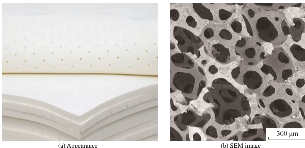
图1 乳胶泡沫材料的结构 Fig.1 Structure of latex foams
