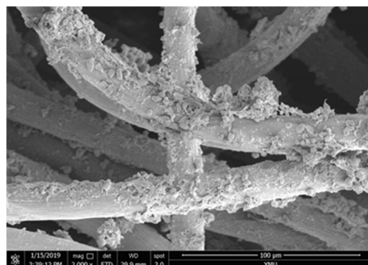
(b) Algae attached on the plain graphite felt
