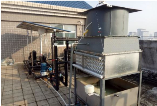
图 1 闭式热源塔热泵系统实物图 Fig.1 Photo of the closed-type heating tower heat pump system
